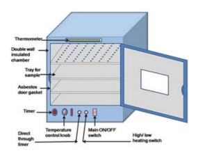
A hot air oven is an essential laboratory equipment that uses to dry heat (hot air) to sterilize laboratory objects and samples. This type of sterilization is also known as dry heat sterilization.
