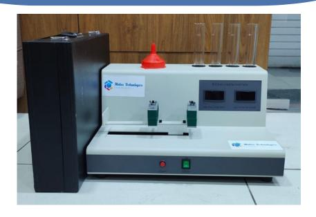
The sand equivalent testing instrument produced by our company is a product designed strictly in accordance with the T0758-2011 Highway Specifications. It is suitable for determining the cohesive soil or impurity content in natural sand, artificial sand, and crushed stone with a maximum aggregate particle size not exceeding 4.75mm (5mm round sieve) to evaluate the cleanliness of the aggregate.
